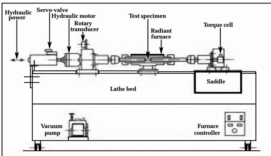
Fig. 3 — Typical torsion tester: a servo-controlled, hot torsion machine mounted on a lathe bed. Shafts and axles are among the parts that should be torsion tested. (Ref. 3)
