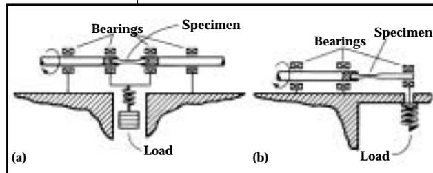
Fig. 5 — Schematics of rotating-beam fatigue testing machines. (a) Four-point loading R.R. Moore testing machine. (b) Cantilever loading machine. (Ref. 6)
