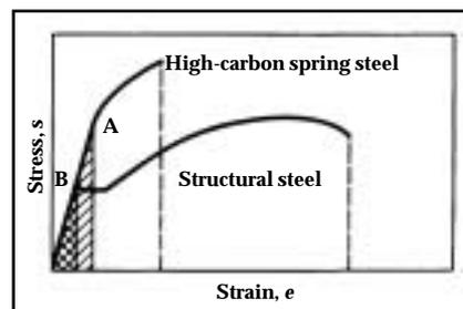
Fig. 8 — Comparison of stress-strain curves for high- and low-toughness steels. Cross-hatched regions represent the modulus of resilience ( $U_R$ ) of the two materials.  $U_R$  is determined by measuring the area under the stress-strain curve up to the elastic limit of the material (point A for the spring steel; point B, the structural steel). (Ref. 9)
