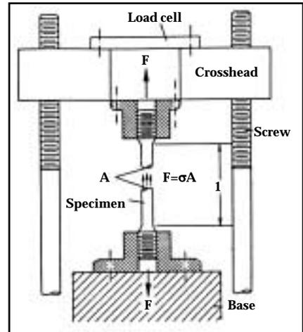
Fig. 1 — Typical tensile tester: a screw-driven electromechanical system. (Ref. 1)
