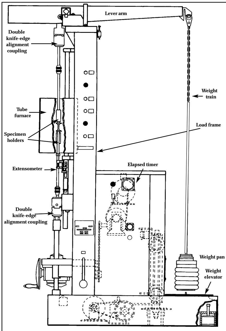
Fig. 6 — Schematic of a test stand used for creep and stress-rupture testing. (Ref. 7)
