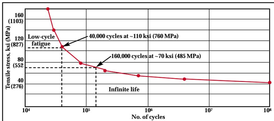
*Fig. 4 — Typical S-N (stress vs. load cycles) curve. A linear reduction in applied stress results in an exponential improvement in fatigue life. (Ref. 5)*
