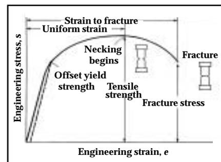
Fig. 2 — Engineering stress-strain curve. Intersection of the dashed line with the curve determines the offset yield strength. (Ref. 2)
